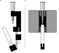
Insert Adapter for MS, LS, and LD Columns in the magnetic field of the SuperMACS™ II Separator (for details, see SuperMACS II data sheets). Place the LS Column in the Column Adapter and the 13 mL collection tube in the lower tube holder.
