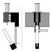
Insert LS Column Adapter in the magnetic field of the VarioMACS™ Separator or the SuperMACS™ Separator (for details, see LS Column Adapter Kit data sheet). Place the LS Column in the LS Column Adapter and the 13 mL collection tube in the tube holder.
