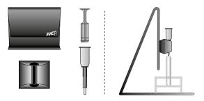
Attach MidiMACS $^{\sim}$  Separator or QuadroMACS $^{\sim}$  Separator to the MultiStand and place LS Column in the separator. Place a collection tube under the LS Column.
